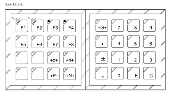
By pressing key F1/F2, the content of PLC address %R0001 is increased/decreased in steps:
